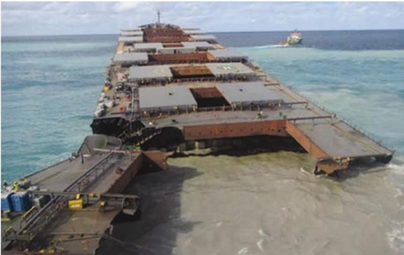
An image depicting the vessel's bow after it separated from the stern (image from the report released by the JTSB)
